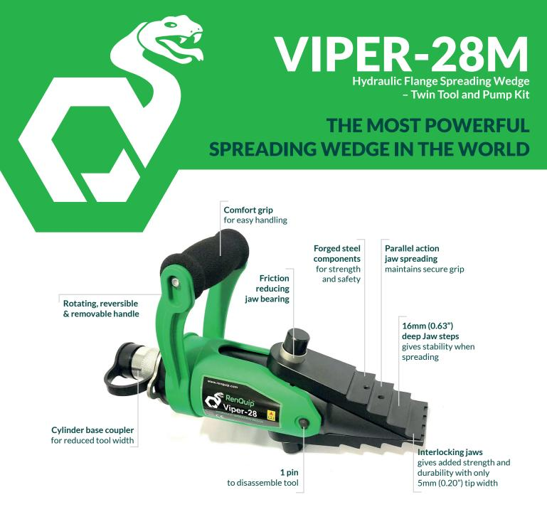
The Viper-28 is RenQuip's latest revolutionary Flange Spreading Wedge – capable of entering a 5mm access gap and producing a spreading force of 277kN (27.7T) per tool yet weighs only 5Kg (11lbs).
